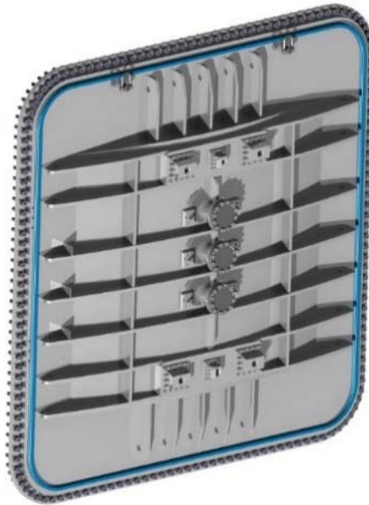
Figure 10: Top Lid bolted on BLV (Similar for DNB Vessel)
